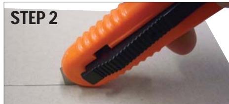
Release blade slider while cutting.
