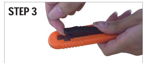
Lift the black slider upwards.
